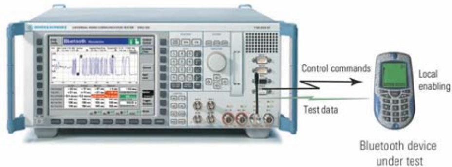
The device under test can be connected to the CMU200 via a RF coupler (antenna) or a cable
